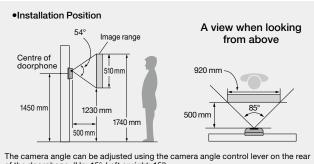
The camera angle can be adjusted using the camera angle control lever on the rear of the doorphone. (Up: 15°, Left or right: 15°)
